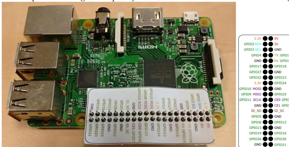
Visit the [http://elinux.org/RPi\\_Low-level\\_peripherals](http://elinux.org/RPi_Low-level_peripherals) webpage for detailed information about individual GPIO pins.
