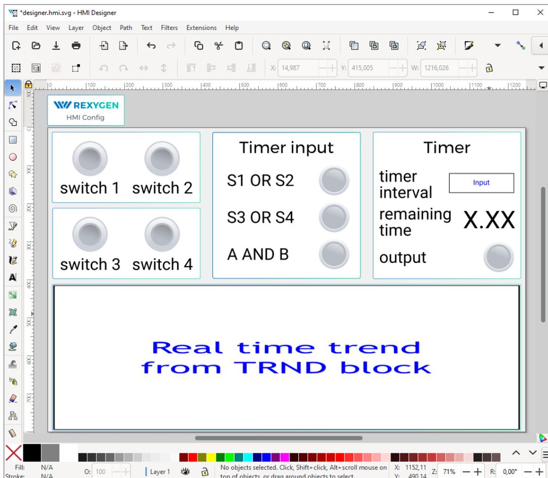
As mentioned earlier, the *\*.hmi.svg* files in the `hmisrc` folder are automatically processed while the project is compiled in the REXYGEN Studio application. The project main file must contain the HMI block with `GenerateRexHMI` parameter set to `on`. This was already set when creating the first project in the manual [1], so you should have everything ready.
