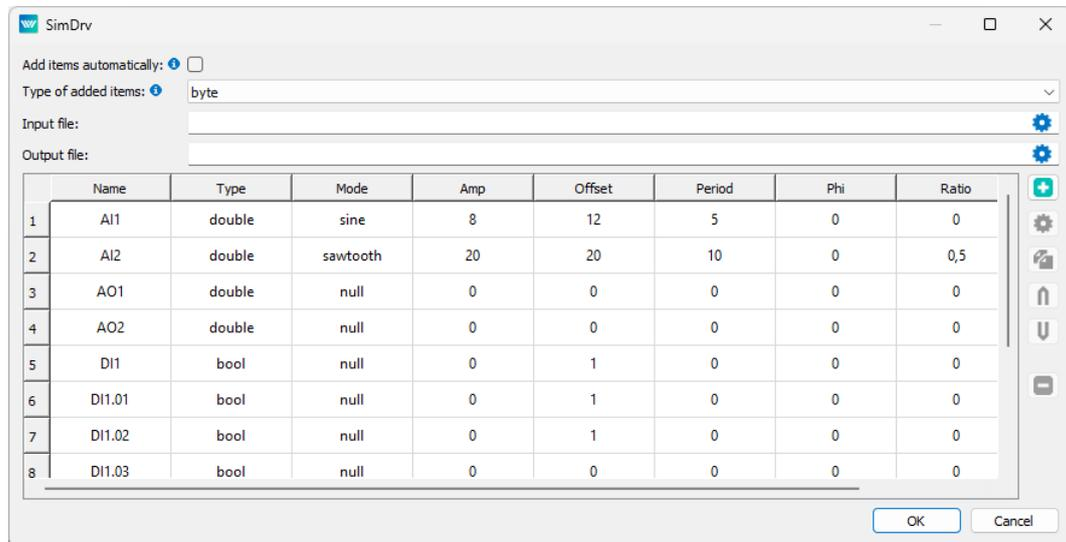
Figure 3.1: Configuration dialog for inputs and outputs
