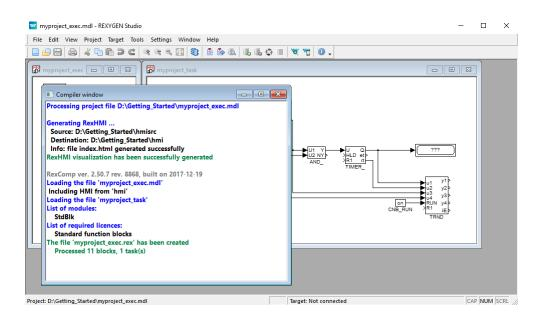
5. After you download the project to the target device, you can access the HMI via web browser. Go to menu *Target/Web Interface* which will open the webpage. Remember the default login credentials: admin with no password.
