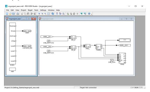
After compiling the project and downloading it to the Raspberry Pi the control algorithm interacts with the physical world. Again it is possible to switch to Watch mode and observe the signals in real-time or analyze the trends of signals. Flip the physical switches and watch the signals.
