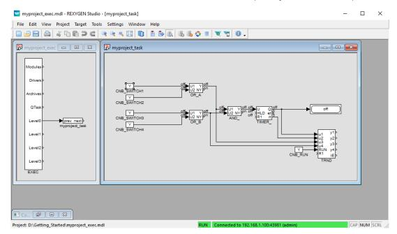
Now it is possible to double-click the CNB\_SWITCH1 block and change the Boolean variable to YCN = on (tick the checkbox and click OK). Once you do the same with the CNB\_SWITCH3 block, the outputs of both OR blocks are on and the Y output of the AND\_ block goes on and the TIMER\_ starts to count down. Observe the rt output.<sup>2</sup> Once the
