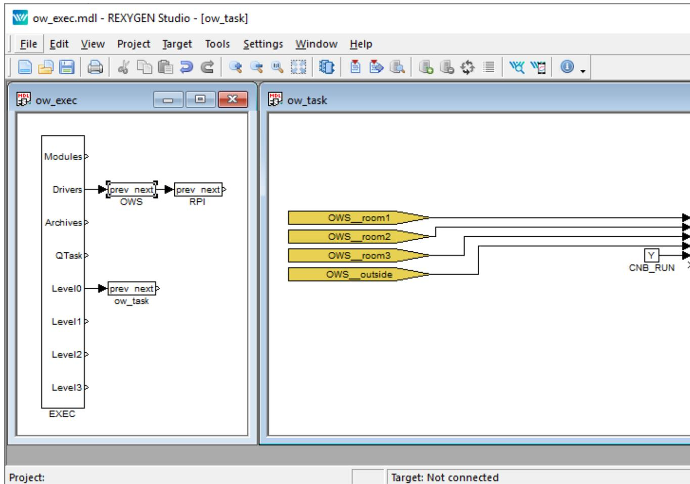
Figure 2.2: Temperature logging based on the `OwsDrv` driver
