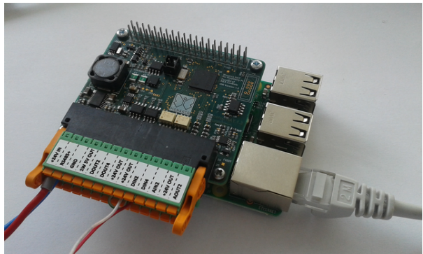
Figure 3.2: Terminal pinout for Monarco HAT.
